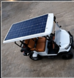
Solar roof golf cart 100 km range, 6.3 kW motor
